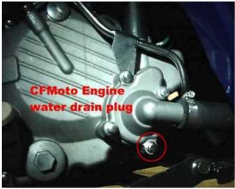
I'm starting with the water, if you have an air cooled scoot, skip to the next section.
