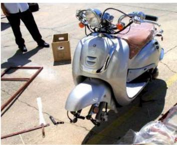
Now it's time to attach the front wheel! If your scoot came with the front wheel attached already, skip to the next step.
