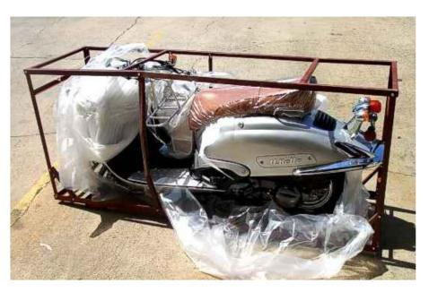
Next, remove all of the bottom bolts on the vertical supports. You may find that the handlebars might be attached to the supports, cut the attachment wires and carefully remove the wire and protective covers on them. The scoot
