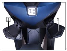
There is a press buckle at the toolbox, which can realize the separation of the box body and the box cover by pressing. Press the box cover again to realize the closure of the box body and the box cover. Use the toolbox(3) only for gadgets.
